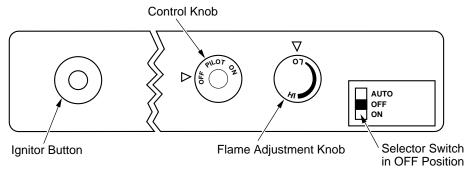
Figure 29 - Control Knob and Ignitor Button Location
